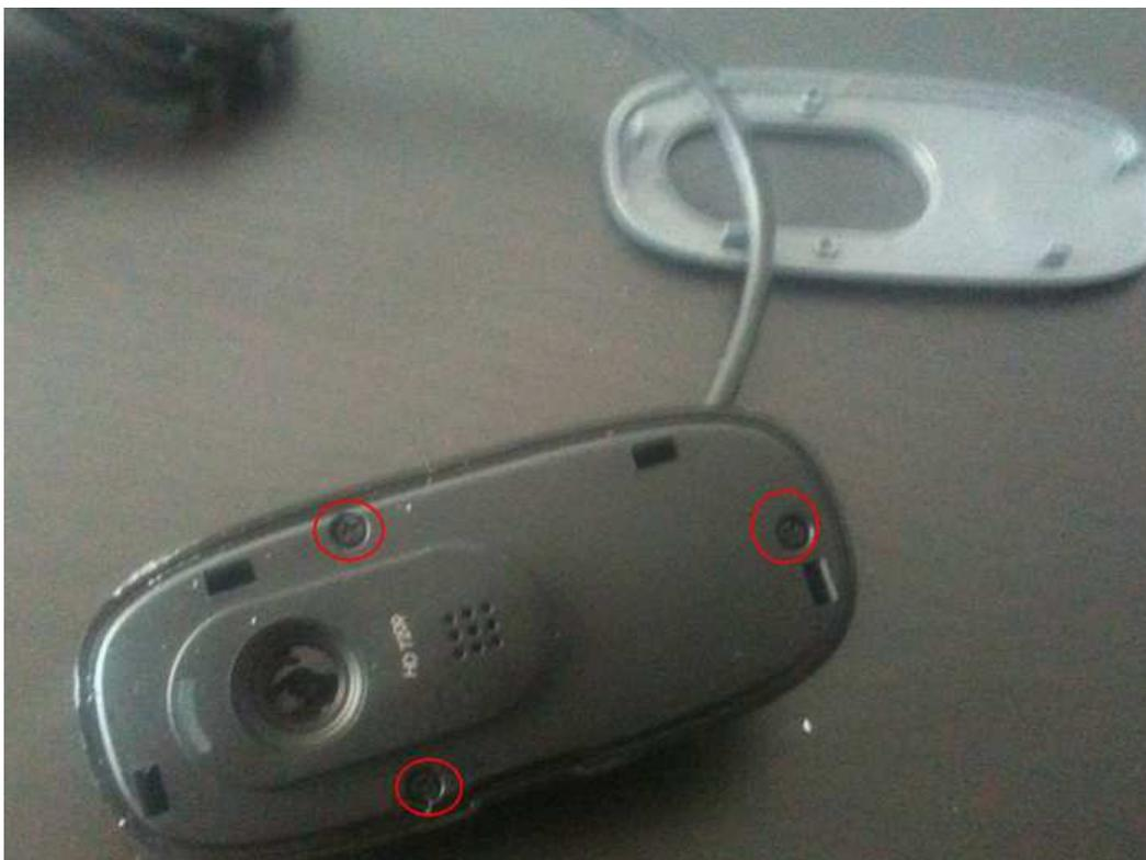
*After you remove the top cover remove the three screws that hold the front of the camera.*
