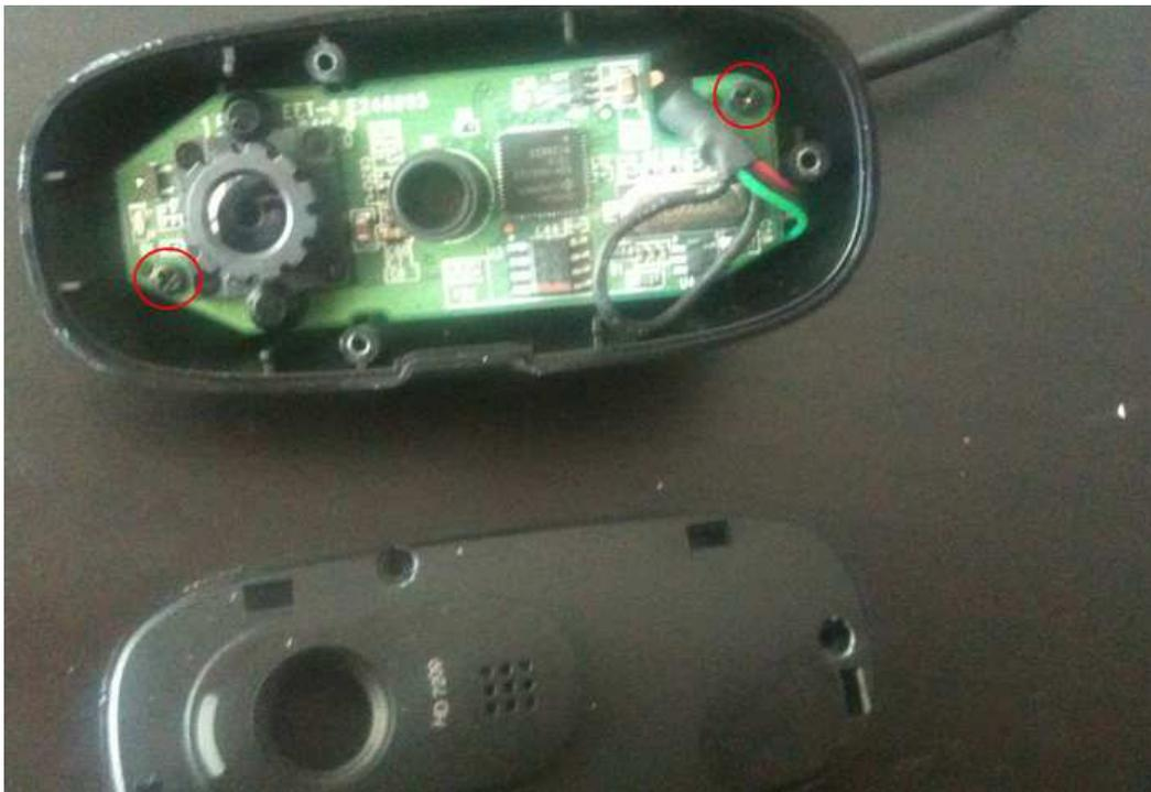
*Remove the two screws that hold the camera board with the case.*
