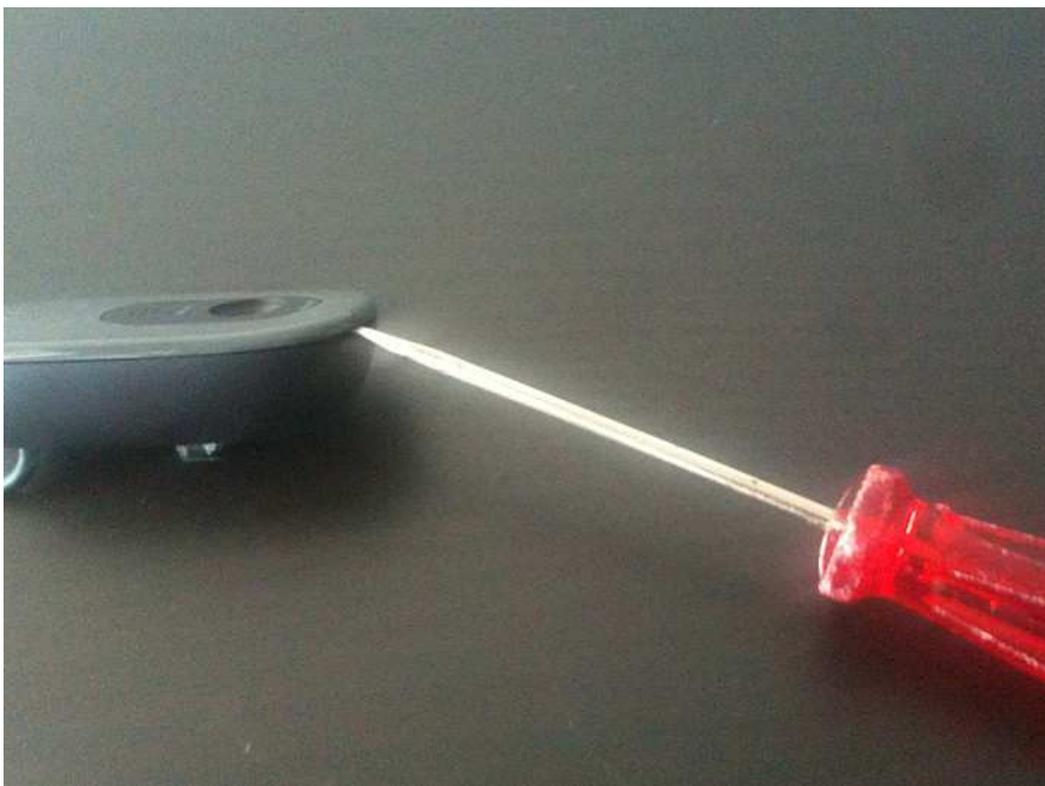
*With the help of a screwdriver carefully lift the top cover.*
