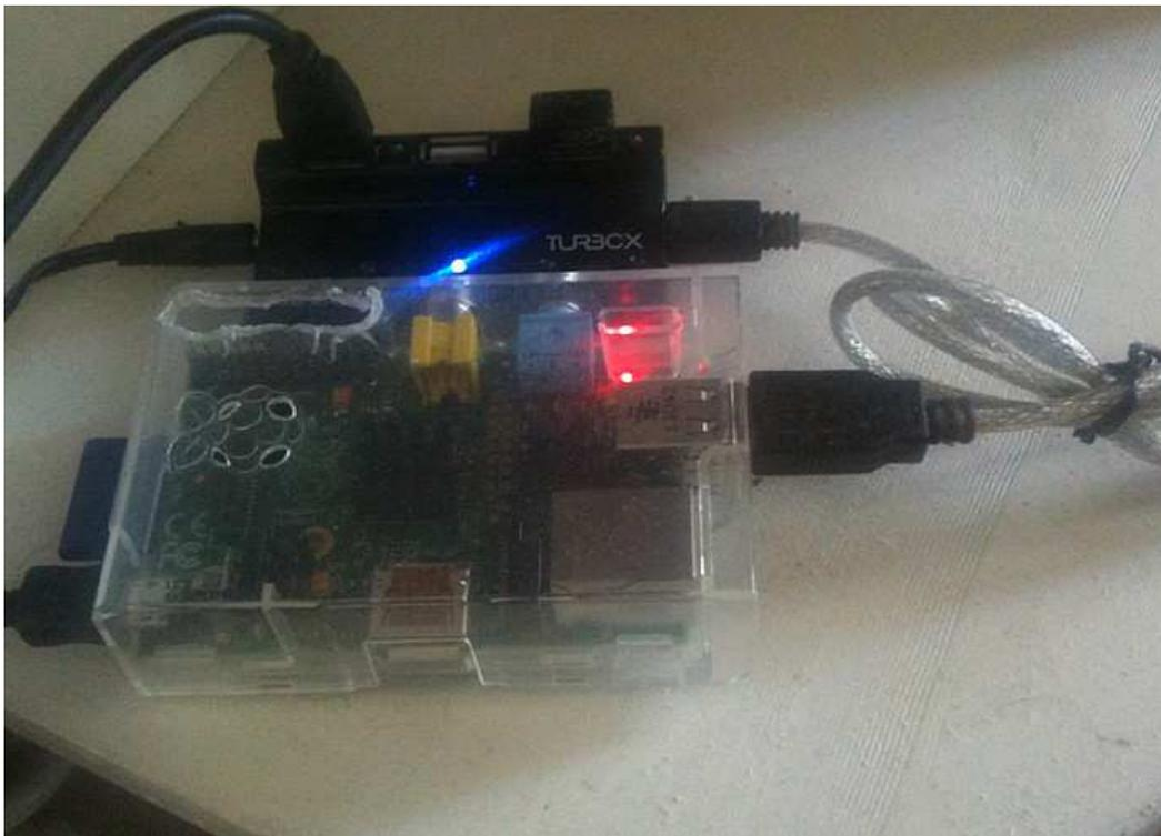
*Connect your webcam to a usb hub with its own external power supply.*
